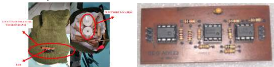
Figure 8. Views: (a) Epy-Tech Outside and Bottom, (b) EEG Circuit Consisting of Amplifier and Filter.
